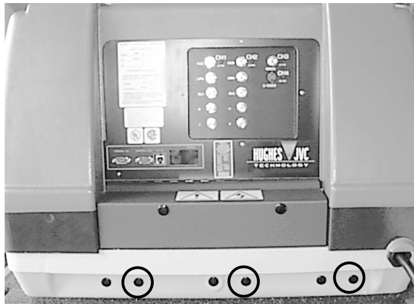
Figure 4-11 CRT Z-Axis Focus Adjustment Rods (circled).
